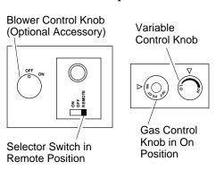
Figure 57 - Setting the Selector Switch, Gas Control Knob, and Variable Control Knob for Remote Operation
